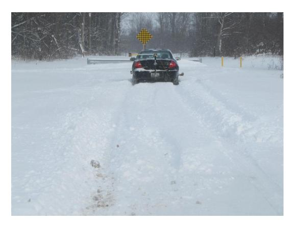
Figure 2: Resultant snow disbursement following braking Test #8 in deep snow.
